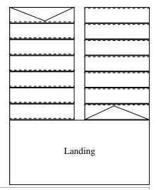
NYS Residential Building Code Landings require a minimum of 36" in direction of travel. 8 1/4" maximum riser height 9" minimum run (tread depth, riser to riser)
